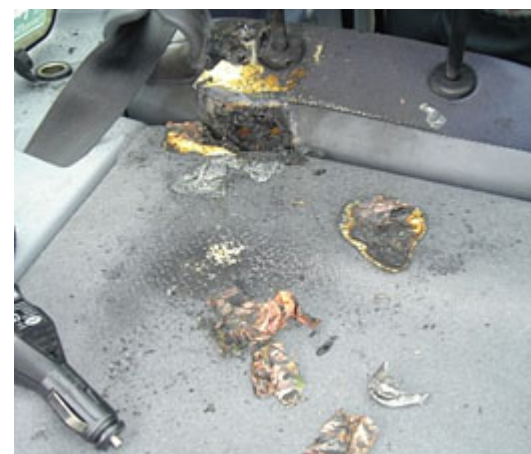
Figure 2: A cell phone with a no-brand battery that vented with flame while charging in the back of a car.
