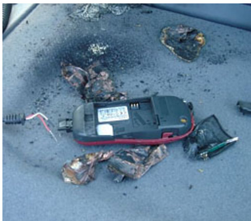
Figure 2: A cell phone with a no-brand battery that vented with flame while charging in the back of a car.
